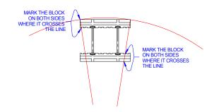
STEP 5 Cut the blocks on the marks, following the angle created by the marks.
