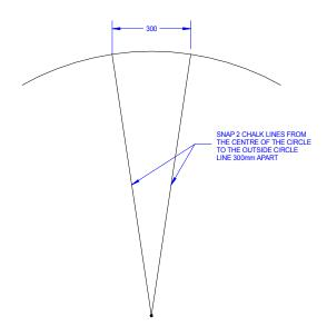
STEP 4 Place one of the 300mm sections on the outside curve line, making sure the outside corners of the block are at the locations of the chalk lines with the curve line
