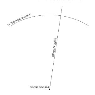
STEP 3 From the intersection of the two lines, measure 300mm and snap a chalk line to this point from the centre of the circle.
